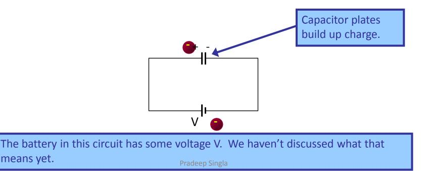
If the external potential is disconnected, charges remain on the plates, so capacitors are good for storing charge (and energy).
