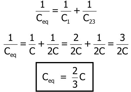
Example: for the capacitor circuit shown,  $C_1 = 3\mu F$ ,  $C_2 = 6\mu F$ ,  $C_3 = 2\mu F$ , and  $C_4 = 4\mu F$ . (a) Find the equivalent capacitance. (b) if  $\Delta V = 12 V$ , find the potential difference across  $C_4$ .
