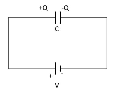
Here's this V again. It is the potential difference provided by the "external potential." For example, the voltage of a battery.
