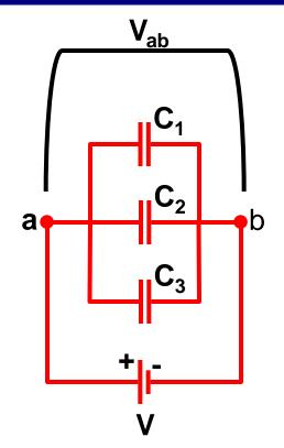
The potential difference (voltage drop) from a to b must equal V.
