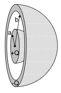
Let  $a \rightarrow R$  and  $b \rightarrow \infty$  to get the capacitance of an isolated sphere.
