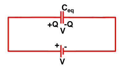
By "equivalent" we mean V is the same as the total voltage drop across the three capacitors, and the amount of charge Q that flowed out of the battery is the same as when there were three capacitors.
