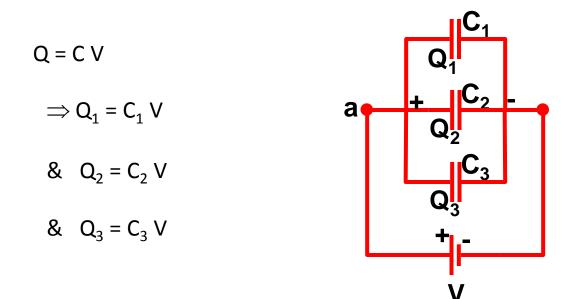
Now imagine replacing the parallel combination of capacitors by a single equivalent capacitor.
