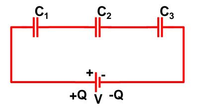
An amount of charge +Q flows from the battery to the left plate of  $C_1$ . (Of course, the charge doesn't all flow at once).
